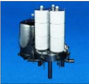
Figure 18 - Like all Zeta Plus housings, this 12ZP9 utilizes an easy to operate, spring loaded sealing system (seen at the top of each filter stack) to ensure reliable cartridge to housing sealing. The housing contains 9 Zeta Plus cartridges and is capable of service flow rates up to 45 GPM (90 HL/hr).
