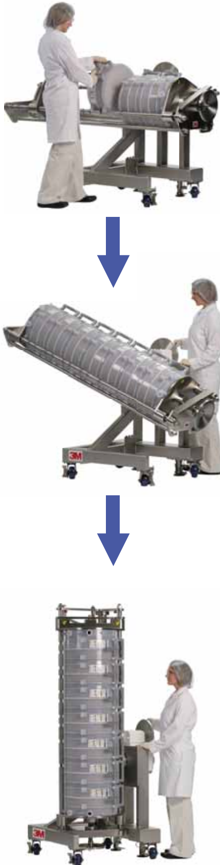
Figure 1. Zeta Plus™ Encapsulated Large Holder Loading Process
