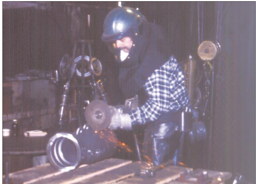
Grinders at U.S. Pipe wear the L-901 Helmet with a wide-view lens that helps to reduce eye injuries.
