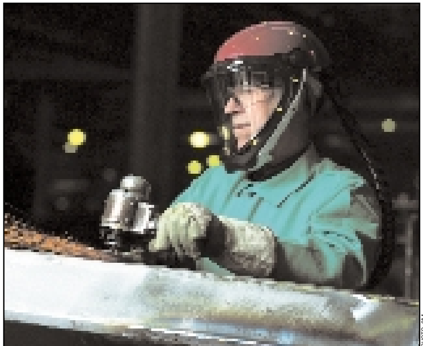
In addition to protecting workers from airborne contaminants, positive-pressure respirators can protect the eyes, face and head, and help guard against heat stress.
